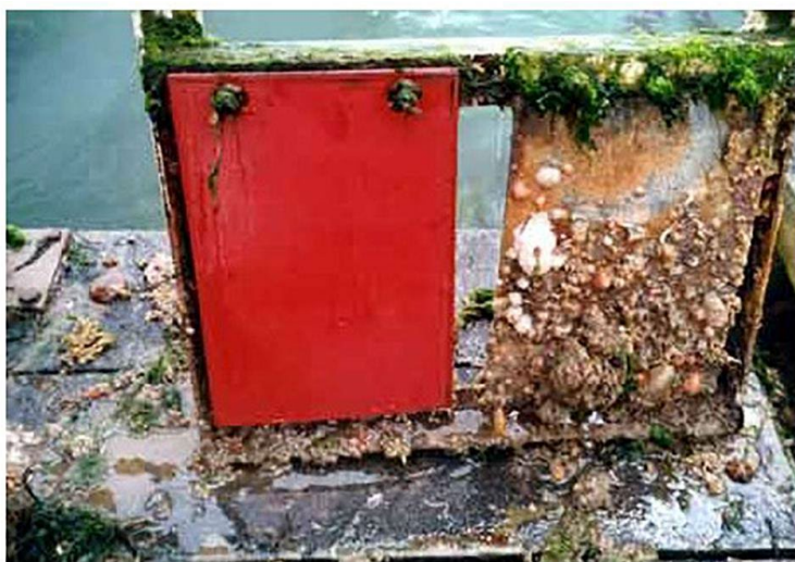
Figure a: TBT has been used as an antifoulant in paint on ship hulls (image from Parmentier et al., 2019)
