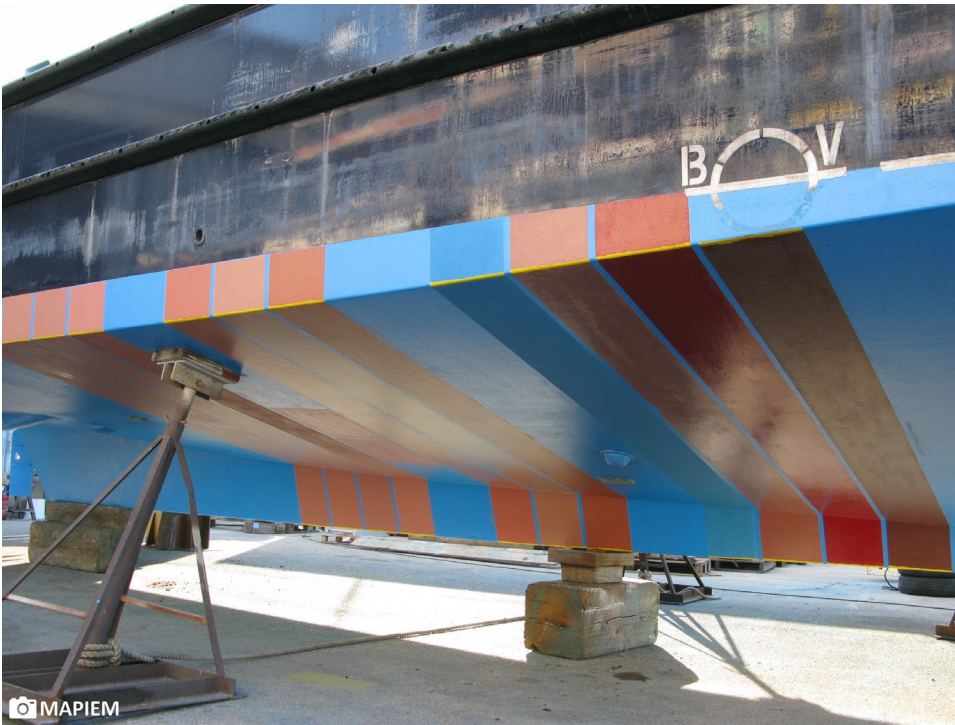
Figure 1: Patch testing antifouling material. © MAPIEM, University of Toulon
