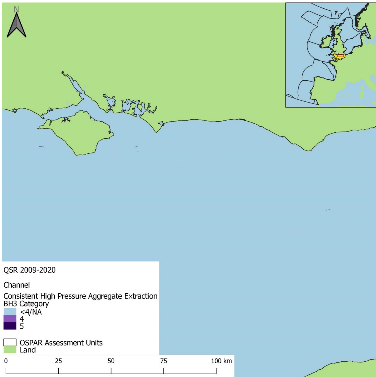
Figure a134: Spatial distribution of consistently high (category 4 or 5) extraction pressure within the 2009 to 2020 assessment period in the Channel assessment period. Grid cells were considered to have ‘Consistent’ pressure if a change in less than three pressure categories was observed within the assessment period.
